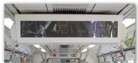
BUSAN METRO HAS INSTALLED A IOT-BASED EVACUATION SYSTEM. SIGNS LIKE THESE TELL WHICH ROUTE IS THE FASTEST AND SAFEST FOR EVACUATION. (IMAGE: MINISTRY OF SCIENCE AND ICT)
